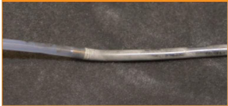
Figure 1: Third-party spliced channel repair
