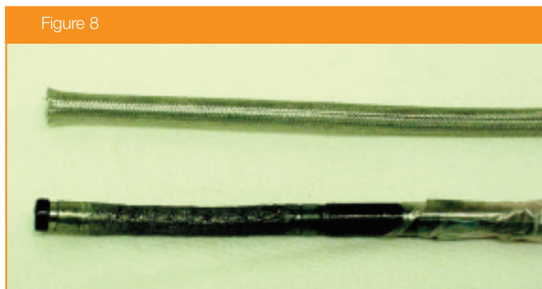
Figure 8: Olympus braided mesh and bending section replacement repair
