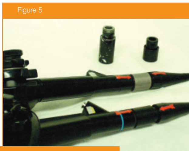
Figure 5: Third-party repair using boot extenders
