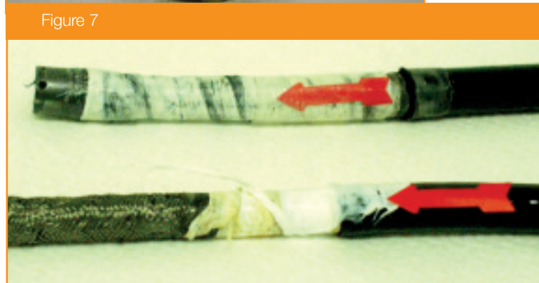
Figure 7: Third-party bending section braided mesh (distal end) band-aid repair
